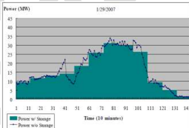
Figure 4.2 Storage Capacity and Time: 5.508 MWh, 2 hours
