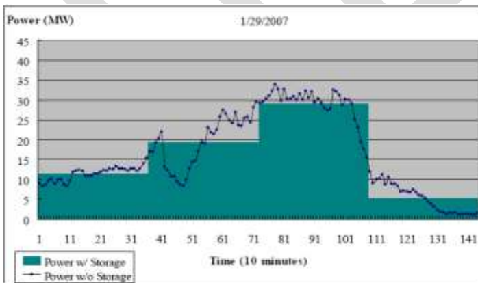
Figure 4.3 Storage Capacity and Time: 16.233 MWh, 6 hours
