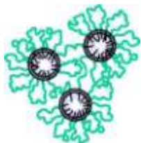
Figure 1-1. The triblock copolymers form loops and bridges on micro emulsion droplets. Dark double circles indicate surfactant layer between two immiscible liquids.
