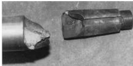
Fig. 4. Failure due to reverse torsional loading [3]
