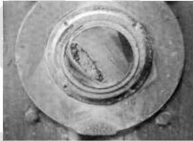
Fig.2. Failure caused by rotational bending [3]
