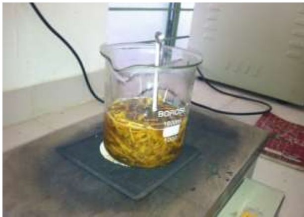
Fig.10: cooking liquor and raw material
