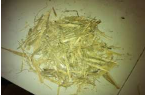
Fig.9: crushed and dried banana stem pieces
