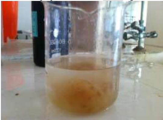
Fig.18:soda pulp after bleaching
