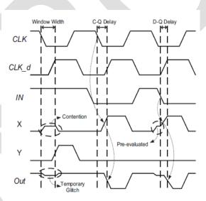
Fig 3: Timing Diagram of CD Logic [7]
