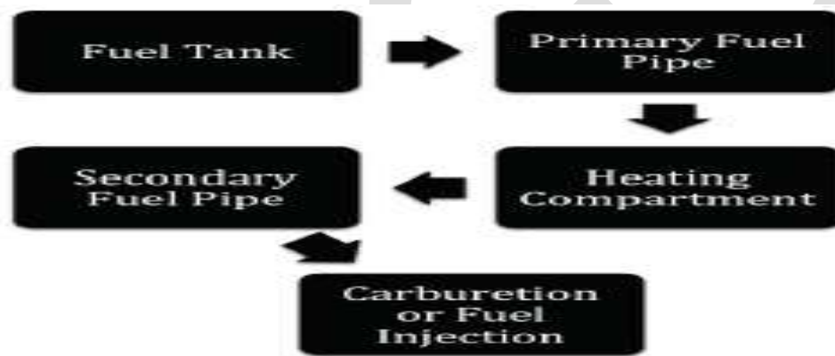
Fig. 3: Block diagram of fuel flow
