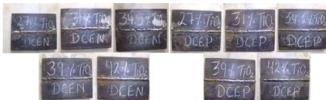
Fig. Weld beads obtained on welding with DCEN and DCEP
