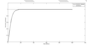
Figure 10- FMPC response (tank 1)
