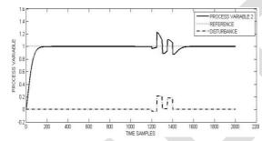
Figure 13- Disturbance rejection
