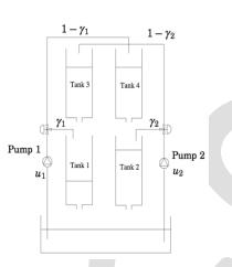
Figure 1 Setup of quadruple tank system
