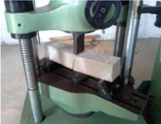
Figure 6: Test on RC beam
