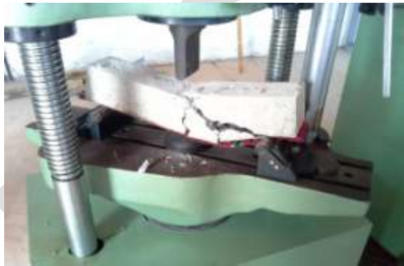
Figure 8: Test on RC beam Retrofitted with coir FRP
