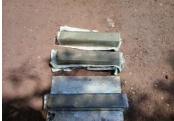
Figure 4: RC Beam Retrofitted with Glass Fibre sheet
