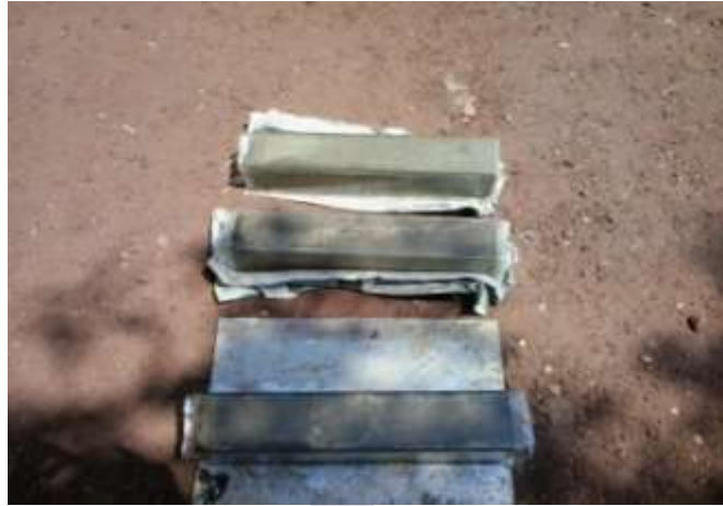
Figure 4: RC Beam Retrofitted with Glass Fibre sheet
