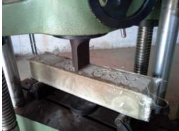
Fig. 7: Test on RC beam Retrofitted with GFRP
