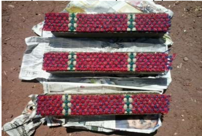
Figure 5: RC Beam Retrofitted with Coir Fibre sheet
