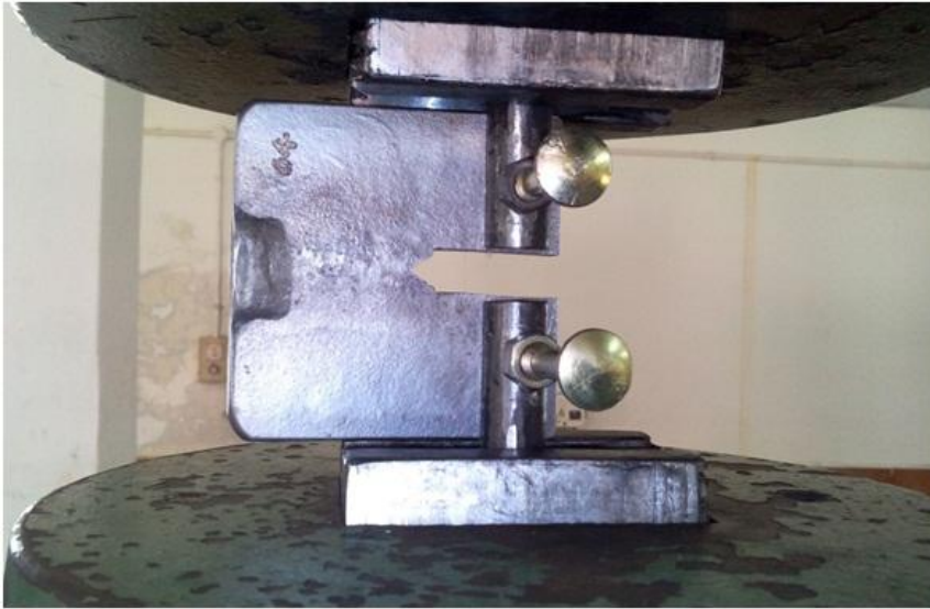
Figure 3 Test Plate with Fixture
