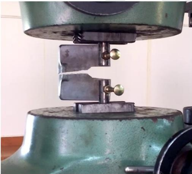
Figure 4 Test Plate after reaching maximum load
