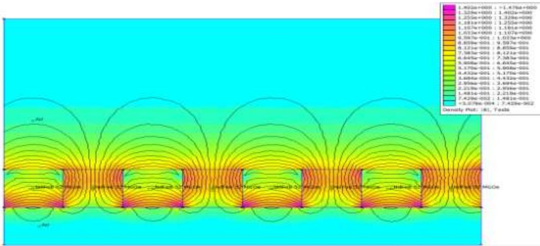
Fig 1.Linear Halbach Arrays
