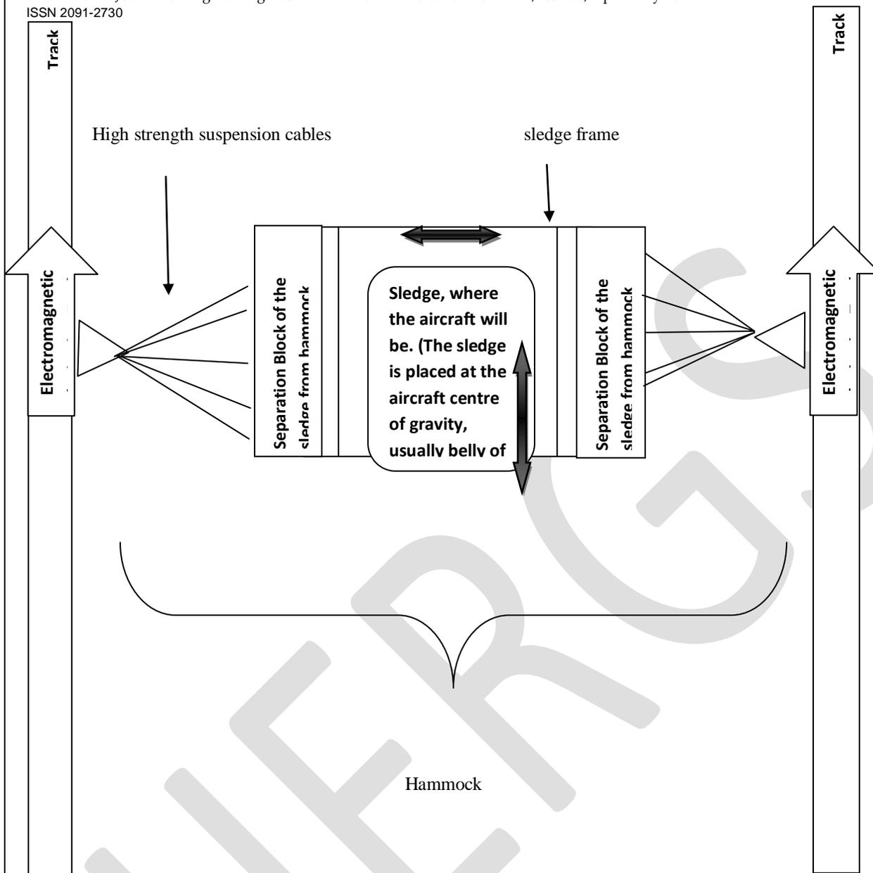
Fig. 2: Basic design concept of magnetic levitation sledge with hammock.
