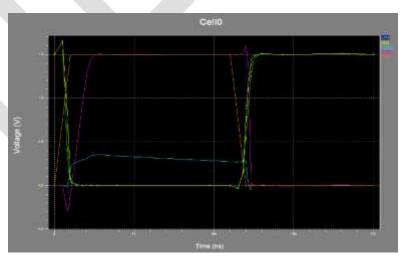
Fig6.2.Conventional double tail Comparator Simulation Results
