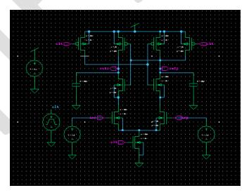
Fig2.1.Schematic diagram of single-tail dynamic comparator.
