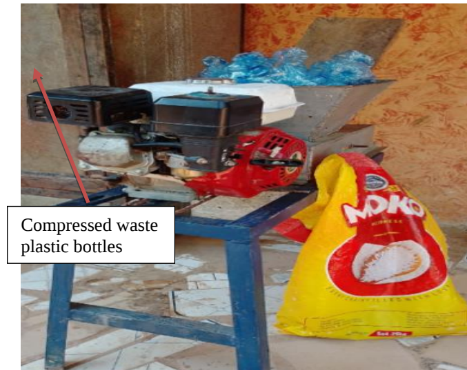
Figure 2: Plastic grinding machine
