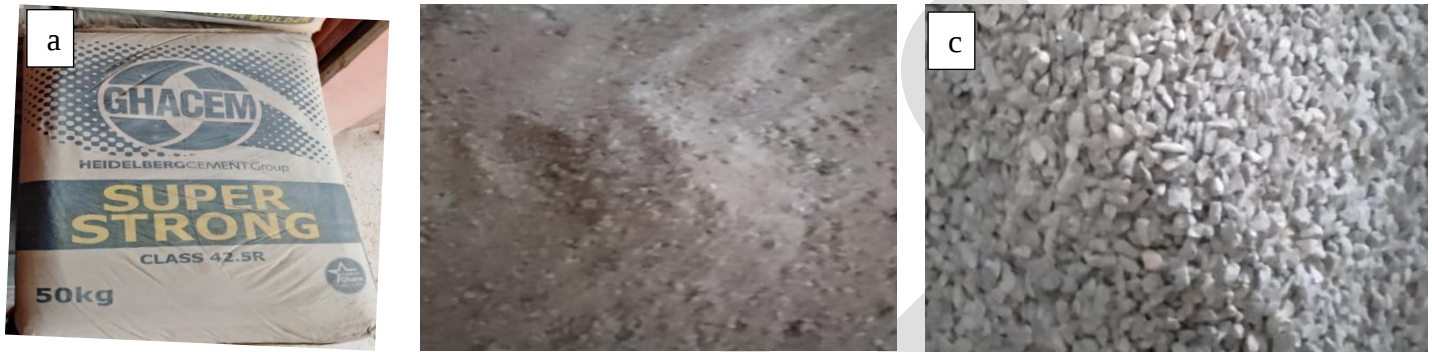
Figure 1: Materials for concrete: (a) cement, (2) fine aggregate, (3) coarse aggregate
